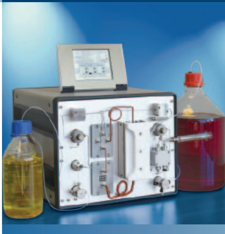
The H-Cube Midi™ reactor was chosen for the purpose because their batch equipment was not suitable and the H-Cube Midi™'s electrolytic hydrogen generation meant it was compatible with their lab without the need for hydrogen facilities.
