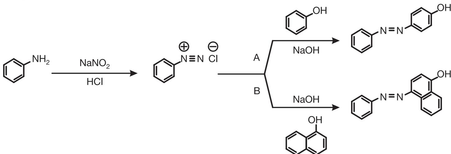
**Scheme 1.** Multistep diazotization and subsequent azo coupling reactions in the IceCube™ flow reactor.
