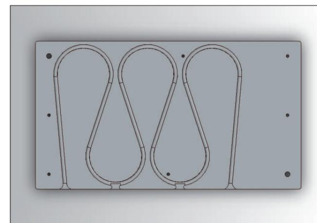
Picture 1. Reactor plate for 1/8''-OD PTFE reactor tubes
