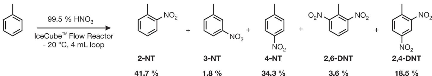
Reaction 2. Nitration of toluene in the the IceCube Flow Reactor
