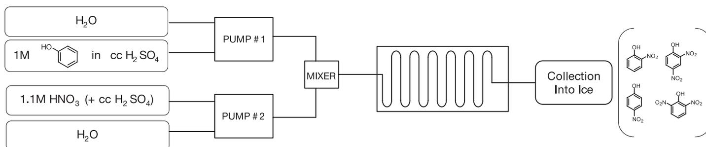
**Scheme 1.** Reaction setup of the IceCube flow reactor for the nitration of phenol
