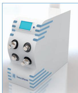
**Pump Module** is made up of 2 rotary piston pumps, which have good chemical compatibility. The pumps are connected to two pressure sensors and 3-way valves, which control the path of reactant or solvent through the reactor. Flow rate: 0.2-4 mL/min. Max pressure: 6 bar
