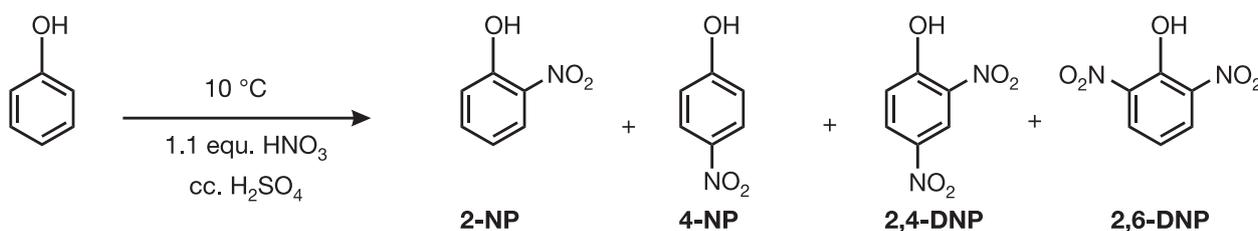
**Reaction 1.** Nitration of phenol in the IceCube flow reactor
