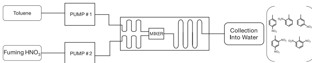
Scheme 2. Reaction setup of the IceCube flow reactor for the nitration of toluene
