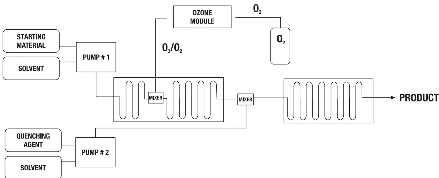
**Figure 2.** Reaction setup of the IceCube flow reactor for ozonolysis
