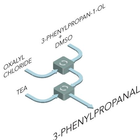
**Scheme 2.** Experimental setup of converting 3-phenylpropan-1-ol to 3-phenylpropanal, utilizing Swern oxidation in the IceCube™ Flow Reactor.
