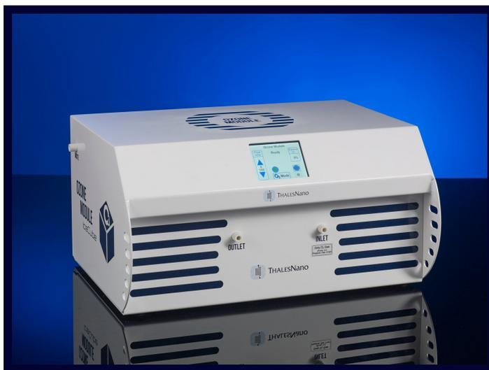
The Ozone Module™ provides a safe and efficient way of generating ozone from oxygen with the oxygen amount precisely controlled through the built-in mass flow controller. This system can also be used as a powerful and compact standalone ozonizer. The Ozone Module™ will need an oxygen generator such as a cylinder to operate.
