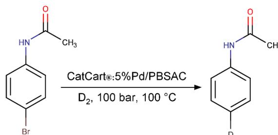
**Scheme 1.:** Deuterodehalogenation of 4-bromoacetanilide with *in situ* generated D<sub>2</sub> reacted over a novel 5% Pd/PBSAC catalyst loaded CatCart®.
