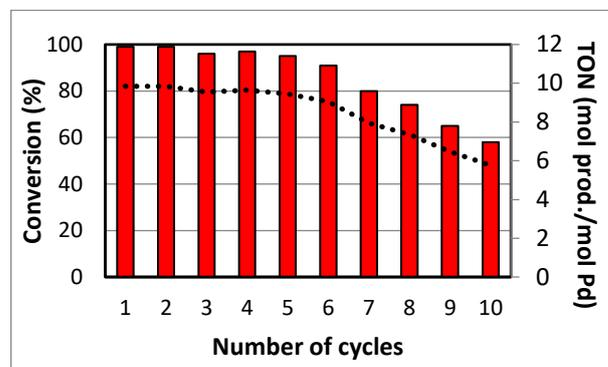
**Figure 1.:** Robustness of the continuous-flow deuterodehalogenation of 4-BAN. The reaction was repeated 10 times on the same catalyst bed. The dashed line shows the TON value for each cycle.
