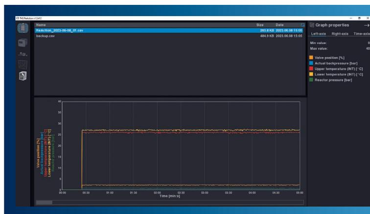
To ensure comprehensive record-keeping and easy data retrieval, the THS ReAction® software features robust data logging capabilities. It automatically collects and stores experimental data, including parameter values, time stamps, and any relevant system events. Researchers can easily access this data for analysis, comparison, and reporting, enhancing the reproducibility and traceability of experiments.
