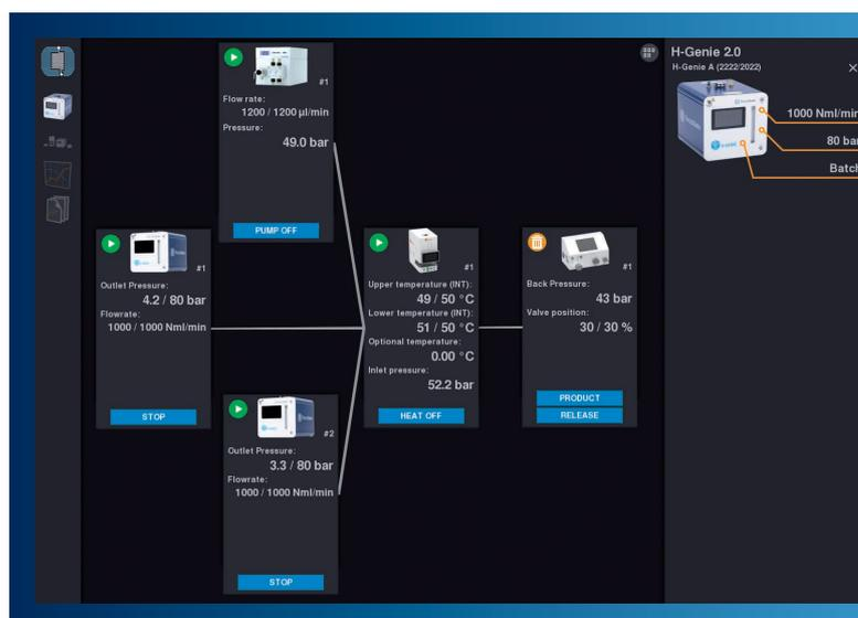
ThalesNano's THS ReAction® software offers a seamless and user-friendly interface to remotely control all laboratory flow chemistry reactor modules. With this feature, researchers can conveniently and efficiently manage various reactor components from a computer, eliminating the need for manual adjustments and increasing experimental precision.
