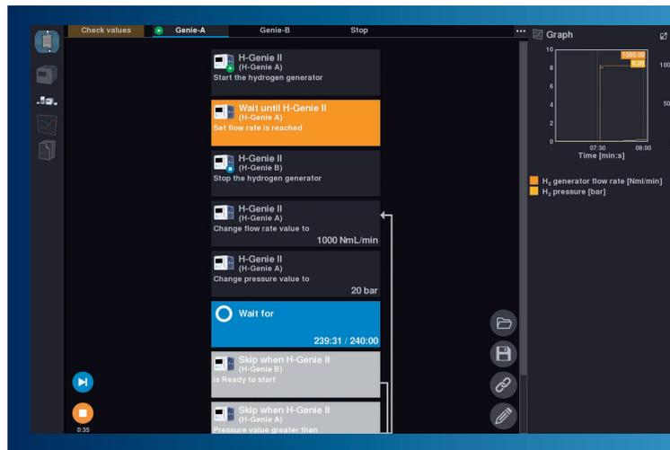
THS ReAction® software incorporates an automated operation mode, which streamlines and optimizes the execution of experimental protocols. Researchers can program the software to follow predefined sequences, execute step-by-step instructions, and adjust parameters automatically at specified time points. This feature not only reduces the risk of human errors but also allows for unattended, long-duration experiments, freeing researchers to focus on other important tasks.
