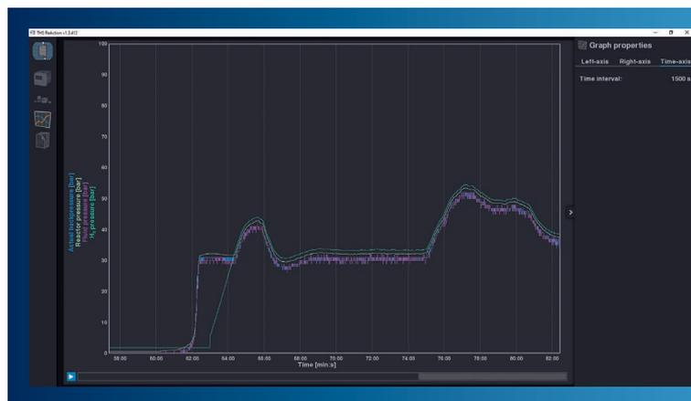
The software provides continuous, real-time monitoring of crucial reaction parameters during the experimental run. Researchers can track variables such as temperature, pressure, and flow rates on a dynamic graphical interface. This immediate feedback facilitates quick decision-making, enabling adjustments or interventions as needed during the course of the experiment.
