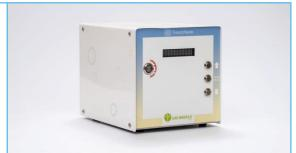
**Pressure Module:** responsible for building the back pressure inside the reaction zone using an automated valve and pressure sensor. It can be controlled remotely and is equipped with an automated pressure regulation mode, as well as an option for easily switching between waste and product collection.
