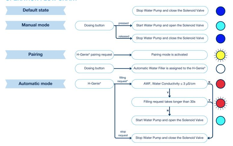
\*the H-Genie® sends water filling request when the upper and the bottom level switches are in down position
